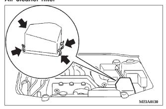
The air cleaner filter will become dirty and loaded with dust during use, and the filtering effect will be substantially reduced. Replace it with a new filter in accordance with the schedule in this manual.
